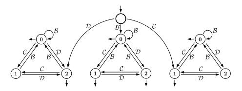
Figure 4: Automaton recognizing non-empty words not containing  $\mathcal{CC}$  or  $\mathcal{DD}$  and not ending with  $\mathcal{C}$  (resp.  $\mathcal{D}$ ) if they start with  $\mathcal{D}$  (resp.  $\mathcal{C}$ ).
