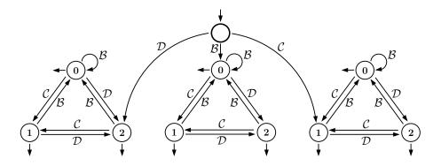
Figure 7: Automaton recognizing words not containing  $\mathcal{CC}$  or  $\mathcal{DD}$ , and reading the first letter separately.
