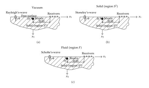
**Figure 1:** Canonical interface models to be solved by means of the indirect boundary element method. (a) Vacuum-solid interface, (b) solid-solid interface, and (c) fluid-solid interface.
