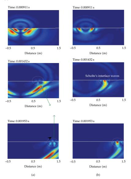
**Figure 6:** Snapshots by IBEM for the complete 2D water-sandstone interface model are shown. A grid of  $51 \times 51$  receivers, spaced using a distance increment of 0.04 m, is required. Column (a) plots the results of pressures in the fluid and displacements in the  $x_1$  direction for the solid, while the column (b) plots pressures in the fluid and displacements in the  $x_3$  direction for the solid.
