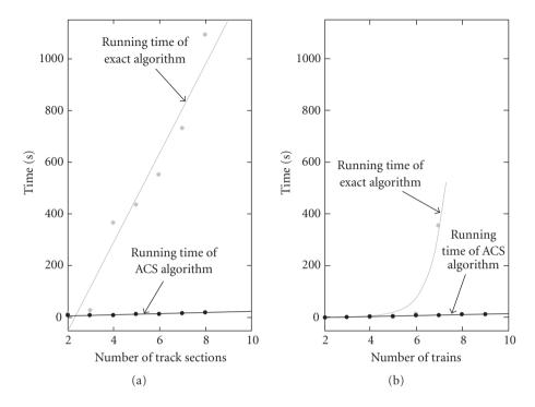
FIGURE 4.1. Run times of solving the train scheduling problems.
