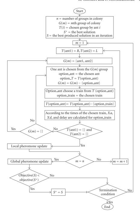
FIGURE 3.2. ACS-TS algorithm flowchart.
