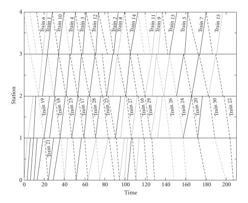
FIGURE 5.1. Time-distance graph of the trains traveling.
