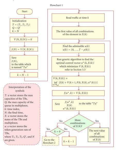
Figure 3.2. Optimal control token-bucket algorithm flowchart (part 1).
