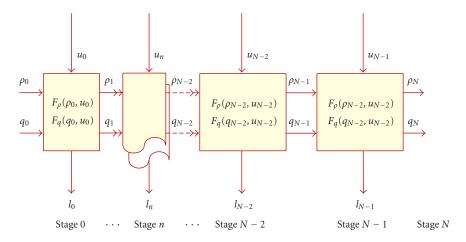
Figure 3.1. Multistage process of token-bucket control problem.
