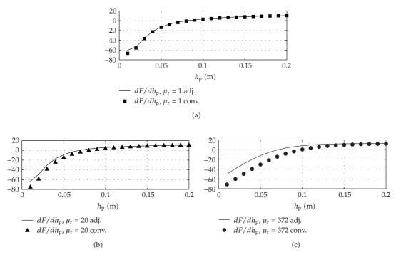
**Figure 6:** Total conventional and adjoint gradients as a function of the height of the passive shield for several  $\mu_r$  and  $\sigma = 5.9 \times 10^6$  S/m (no active shield).
