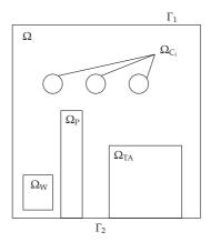
Figure 2: Domain  $\Omega$ .  $\Gamma_2$  is the bottom horizontal border of  $\Omega$  and  $\Gamma_1$  is the rest of the border of  $\Omega$ ;  $\Omega_W$  is the workpiece;  $\Omega_P$  is the passive shield;  $\Omega_{TA}$  is the target area;  $\Omega_{C_i}$  are the compensation coils of the active shield.
