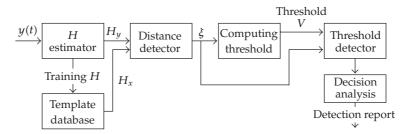
Figure 3: System diagram.
