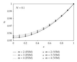
**Figure 2:** Dimensionless temperature distribution for convective-conductive parameter N = 0.1.
