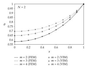
**Figure 5:** Dimensionless temperature distribution for convective-conductive parameter N = 2.
