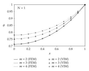
**Figure 4:** Dimensionless temperature distribution for convective-conductive parameter N = 1.
