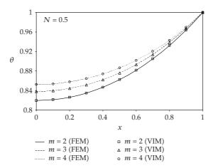
**Figure 3:** Dimensionless temperature distribution for convective-conductive parameter N = 0.5.
