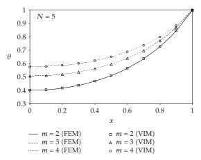
**Figure 6:** Dimensionless temperature distribution for convective-conductive parameter N = 5.
