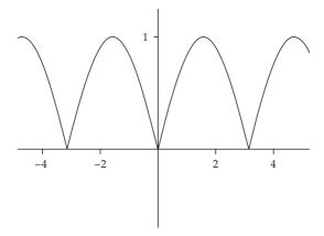
Figure 1: Full-wave rectified sinusoid.
