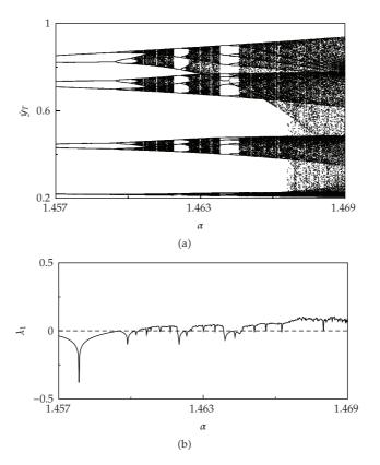
**Figure 7:** Bifurcation diagram of velocity  $\dot{y}_T$  as a function of the amplitude excitation  $\alpha$  for r = 0.683. (b) The largest Lyapunov exponents,  $\lambda_1$ , for attractors of the bifurcation diagram.
