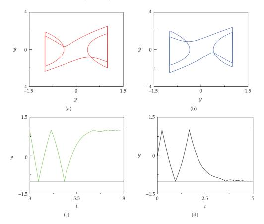
**Figure 3:** Phase portrait of velocity versus displacement of two coexisting periodic attractors (a) and (b). Time histories of two equilibrium points (c) and (d). For the control parameters  $\alpha$  = 3.2 and r = 0.8.
