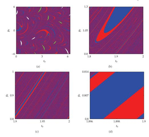
**Figure 4:** Basins of attraction and successive magnifications for the parameters  $\alpha$  = 3.2 and r = 0.8, varying initial conditions  $\dot{y}_0$  and  $t_0$  with  $y_0$  = 0. Basins in red and blue for the two coexisting attractors were shown in Figures 3(a) and 3(b) basins, in green and white for the two equilibrium points were shown in Figures 3(c) and 3(d).
