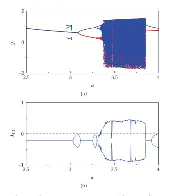
**Figure 2:** (a) Bifurcation diagram showing coexisting attractors. Velocity  $\dot{y}_T$ , for a stroboscopic map, as a function of the amplitude excitation,  $\alpha$ , for r = 0.8. (b) The Lyapunov exponents,  $\lambda_{1,2}$ , for the attractors plotted in blue.
