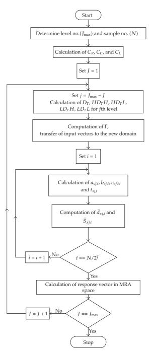
Figure 2: Flowchart of nonsinusoidal steady-state analysis.
