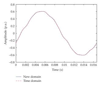
Figure 4: I<sub>Util</sub> waveform comparison of the time and new domain simulations.
