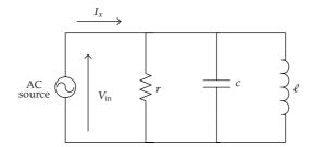
Figure 1: Parallel RLC circuit.
