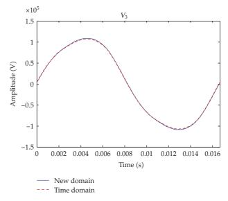
**Figure 7:** Load Voltage  $(V_3)$ : new proposed domain and time domain.
