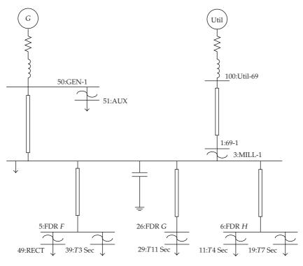
Figure 3: The 13-bus test system.
