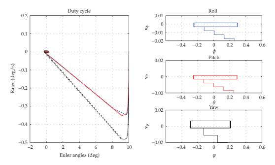
Figure 6: Duty cycle response for stabilization during a short slew maneuver.
