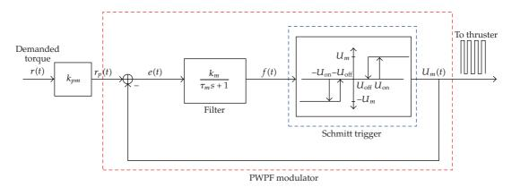
Figure 3: Pulse-width pulse-frequency (PWPF) modulator.
