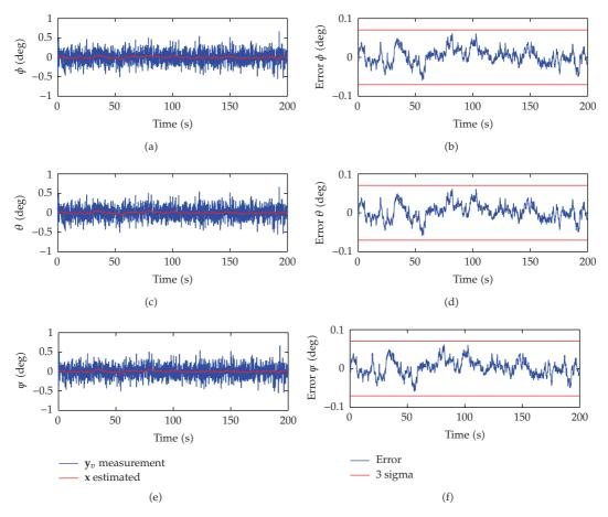
Figure 4: Filtering of the measurement data.
