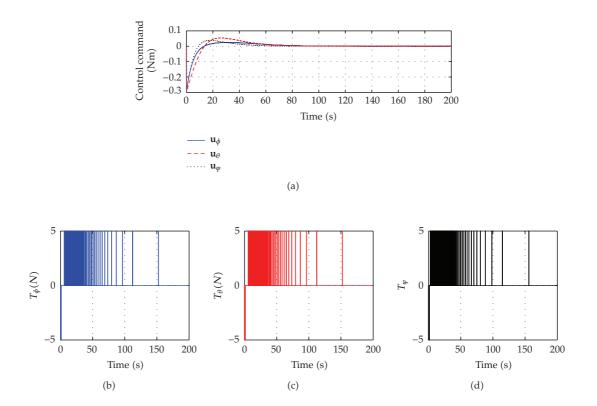
Figure 7: Control command and PWPF modulation during the slew maneuver.
