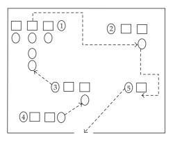
**Figure 2:** M/M/1 queues of the products/semiproducts in a job shop ( $\Box$  represents a server  $\bigcirc$  represents a manufacturer of a semiproduct).
