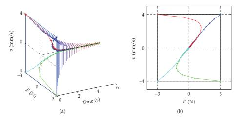
**Figure 3:** (a) 3D representation of the exponentially contractive set  $X_r^1(t; 0)$ . (b) State-space portrait. The same four trajectories as in Figure 2.
