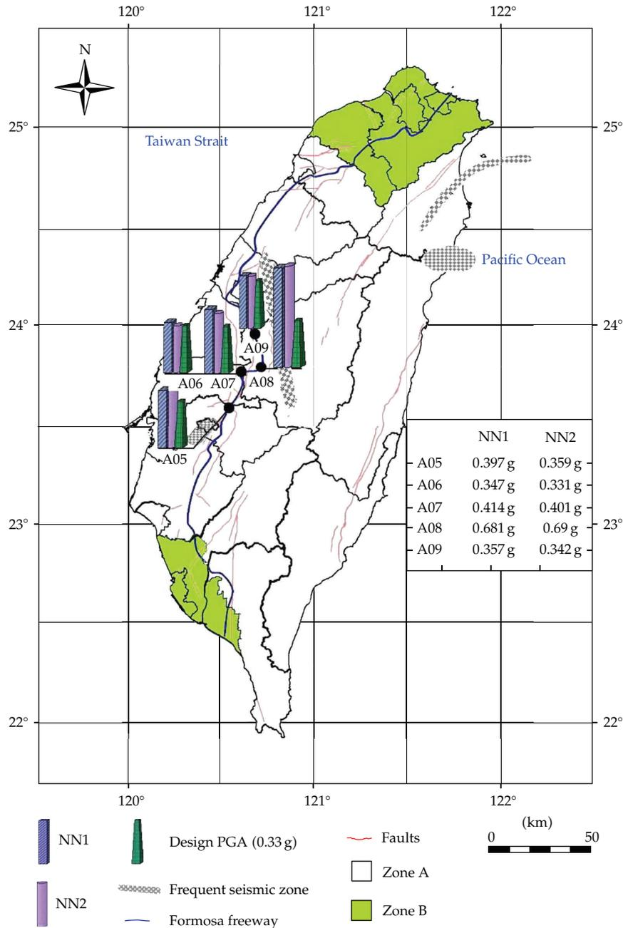
Figure 7: Location of potentially hazardous bridges and estimated horizontal PGAs.
