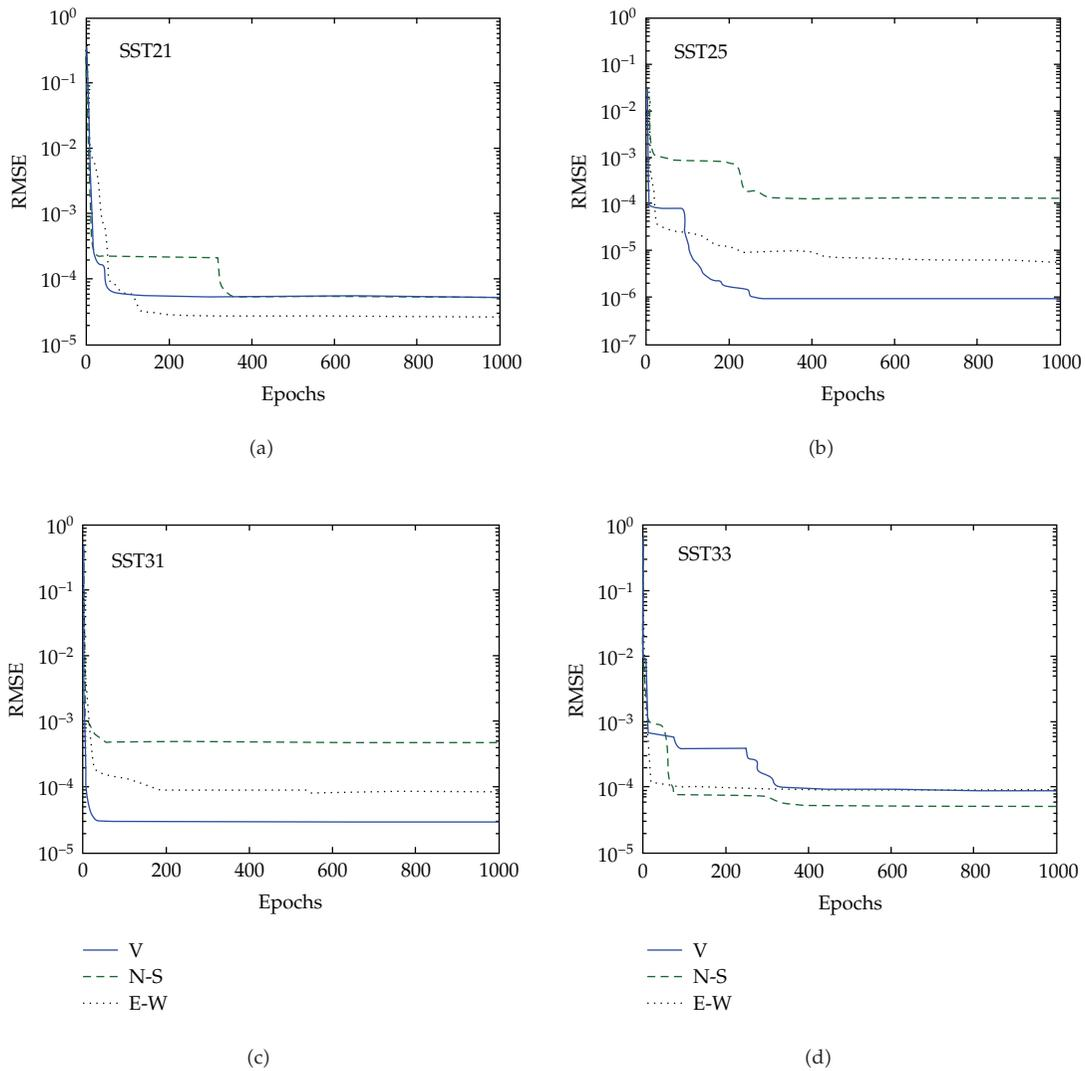
**Figure 3:** Convergence tendency of root mean square error versus epochs for each of checking station around bridge A09.
