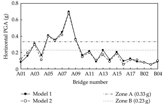
Figure 6: Comparison of horizontal PGA estimations versus seismic design values.
