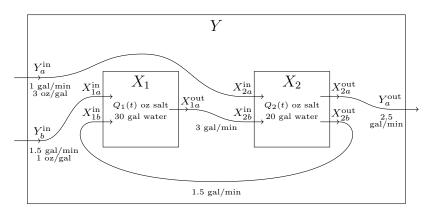
Figure 9: A dynamical system from Boyce and DiPrima interpreted over a wiring diagram  $\Phi = (X_1, X_2; Y; \varphi)$  in  $\mathcal{O}\mathbf{W}$ .
